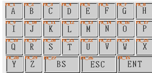
An ASCII keypad consisting of A~Z, BS, ESC and ENT.
